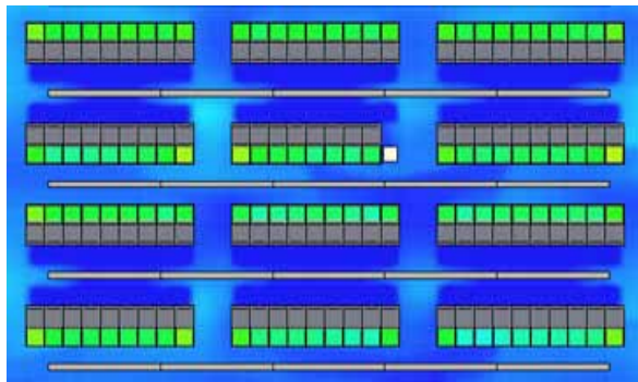
Alternating “hot” and “cold” aisles minimizes unwanted mixing of hot air around the cabinets
